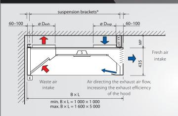
Note: Hoods with a length of L > 3000mm are always supplied with 2 outlets e, and i, placed at 1/4 of the length from the edges.
