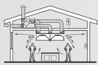
The air intake of the VARIANT series hoods is provided by stainless steel outlets. Each outlet can be easily directed.
